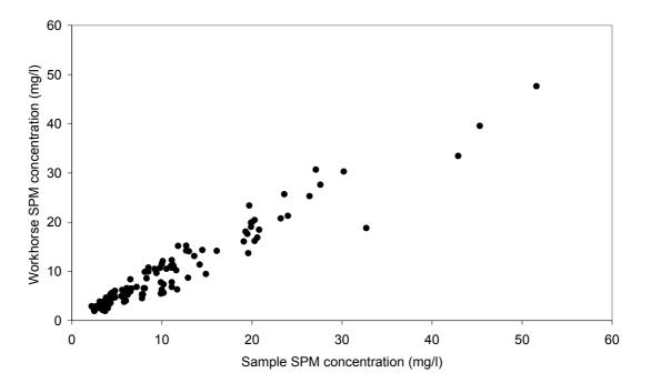
Fig. 2. Calibration of the boat-mounted ADCP (Workhorse). SPM concentration estimates obtained from instruments backscatter data and corresponding water sample measurements (Oct 2004 – Jan 2005).
