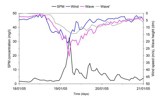
Fig. 7. Time series of average SPM concentration along the vertical profile in the mid-channel of the Lido inlet. Wind speed and significant wave height offshore (Wave) and at the Lido inlet (Wave') are superimposed.
