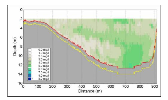
Fig. 3. Distribution of SPM concentrations across the A-A' section in the early flood phase. Transect acquired on January 17<sup>th</sup> 2005 at 13.57 UT.
