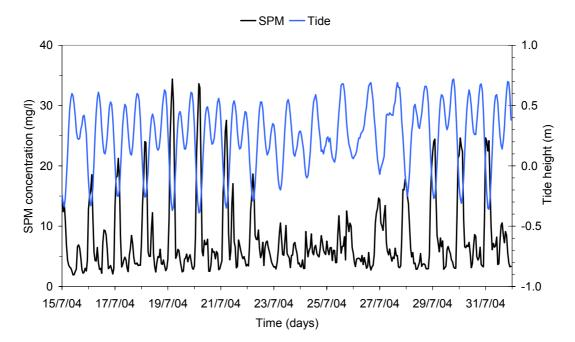
Fig. 6. Extract of the time series of average SPM concentration along the vertical profile in the mid-channel and tide height at the Lido inlet.
