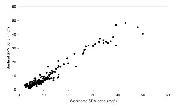
Fig. 5. Calibration of the bottom-mounted ADCP (Sentinel). SPM concentration estimates obtained from the current meter and corresponding indirect estimates provided in the period Jul 2004 – Jan 2005 by the boat-mounted ADCP (Workhorse).
